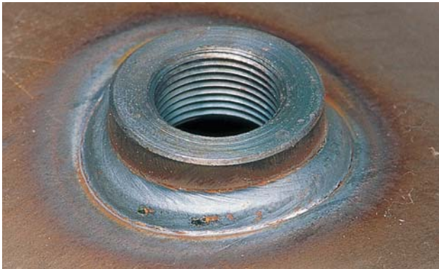
Spatter free welding in Synergic Pulse mode.
