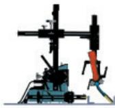
The Moggy performing a fillet weld using a template, guide or fence positioned parallel to the work piece. The actual workpiece is often used as the guide.
