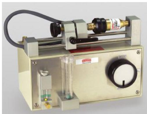
Safety devices have to be tested every year as detailed below. Without changing of position flow rate comparison checks can be made. Additionally the function of the pressure sensitive valve can be checked.
