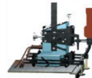
Adjustable height guide roller assemblies are available to track joints with a vertical member higher or lower than the set height of guide roller wheels.
