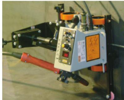
The Gullco Moggy friction drive travel carriage is designed to perform Horizontal Fillet Welding, Lap Welding and Butt Welding. It can be fitted with a Gullco Compact Oscillator to perform multi-pass welding. These operations can be performed on horizontal fillets with a minimum radius of 39 in. (1 meter) and up to a 30° incline.
