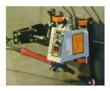
The Gullco Moggy friction drive travel carriage is designed to perform Horizontal Fillet Welding, Lap Welding and Butt Welding. It can be fitted with a Gullco Compact Oscillator to perform multi-pass
